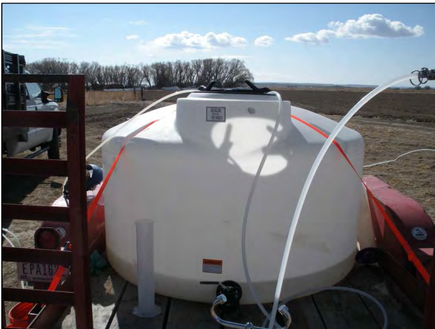
Figure D2. Photograph of flow of water to purge water disposal tank at MW02.
