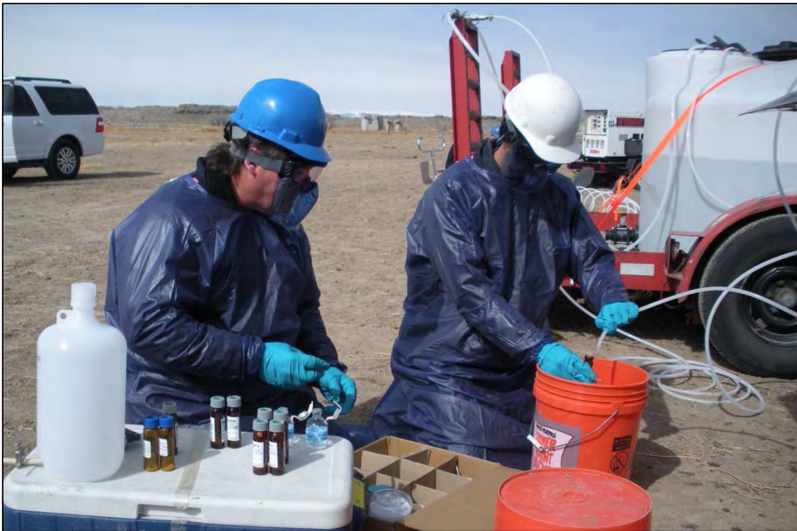
Figure D5. Photograph of sampling at MW02. The sample train was split prior to entry into purge water disposal container.
