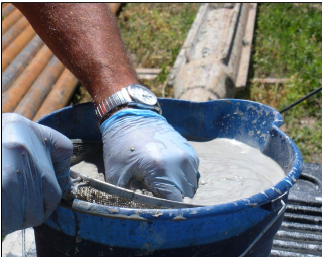
Figure C18. Photograph of removal of mud from cuttings at MW02.
