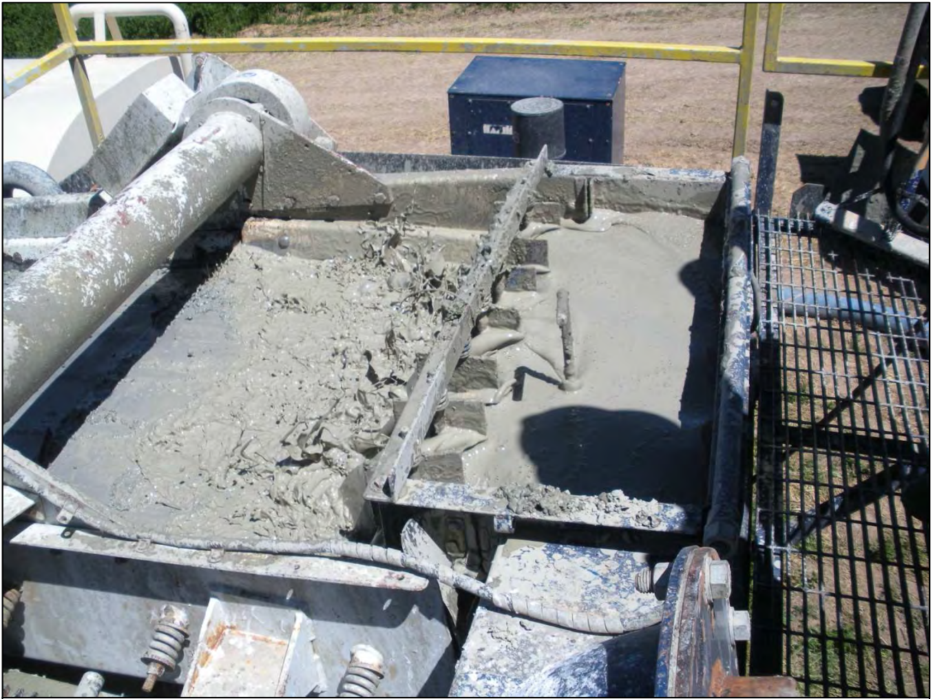
Figure C13. Photograph of shakers separating mud from cuttings at MW02.
