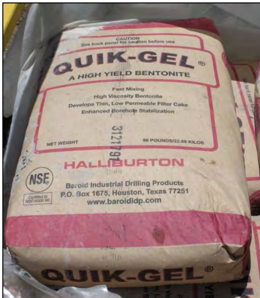
Figure C6. Photograph of Quik-Gel bentonite (Halliburton) used to create mud for drilling.
