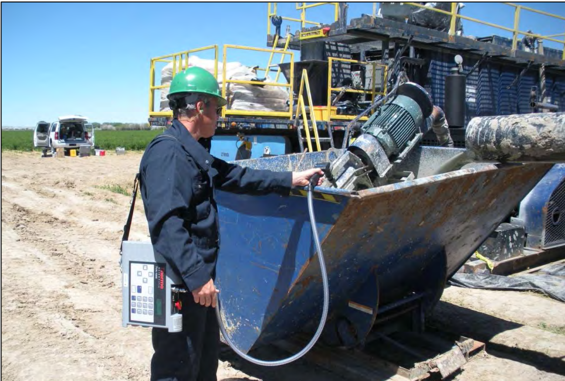
Figure C10. Photograph of monitoring of mud and cuttings using a Thermo Scientific TVA-1000B FID/PID at MW02.
