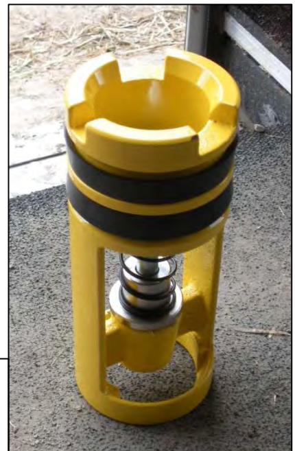
Figure C3. Photograph of blowout preventer for drillstem.
