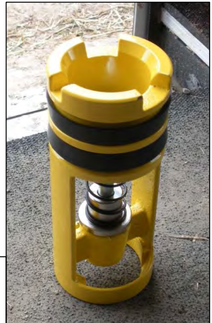
Figure C3. Photograph of blowout preventer for drillstem.
