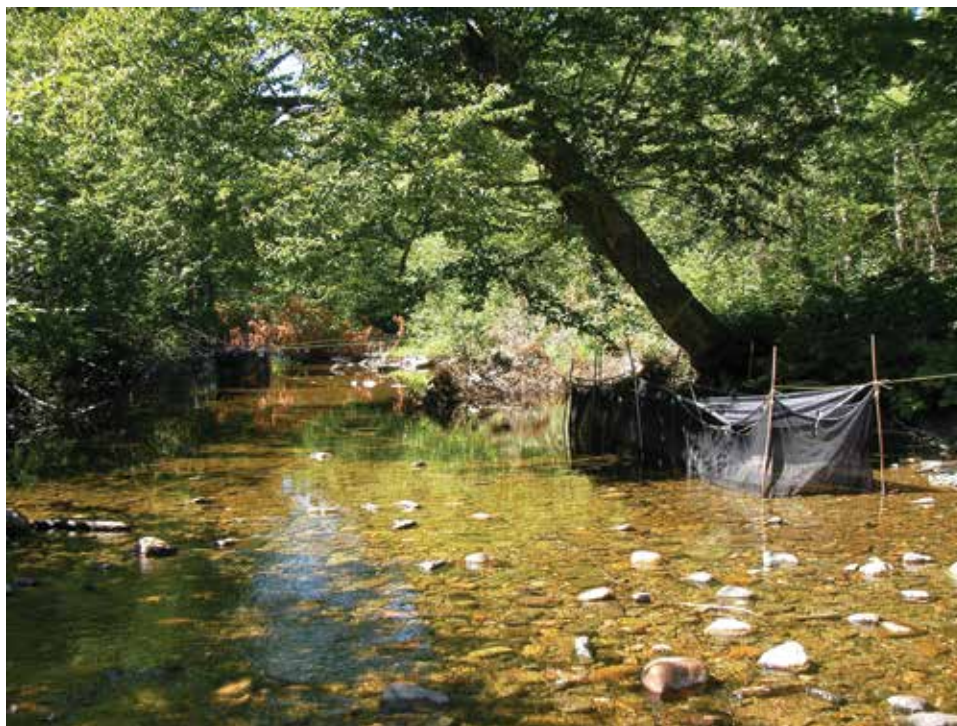
Photo 2. Mesh enclosures anchored in the Catamaran Brook, New Brunswick. Enclosures can be stocked with tagged salmon and allow for long-term studies of behavior under natural conditions. Photo Credit: K. K. Elvidge.
