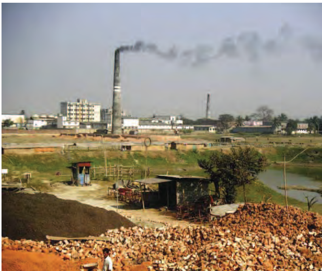
Traditional brick kilns in South Asia are a major source of black carbon. Improved kiln design in this region is significantly reducing emissions.
