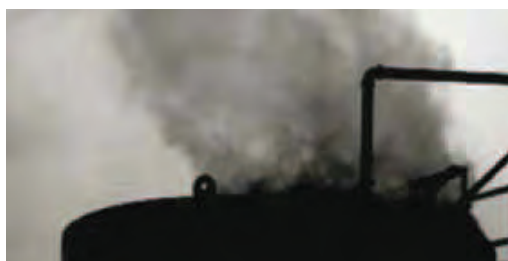
To the naked eye, no emissions from an oil storage tank are visible (left), but with the aid of an infrared camera, escaping CH 4 is evident (right).
