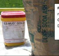
**Figure C7.** Photograph of mud additives EZ Mud Gold (Halliburton) and Dense Soda Ash.
