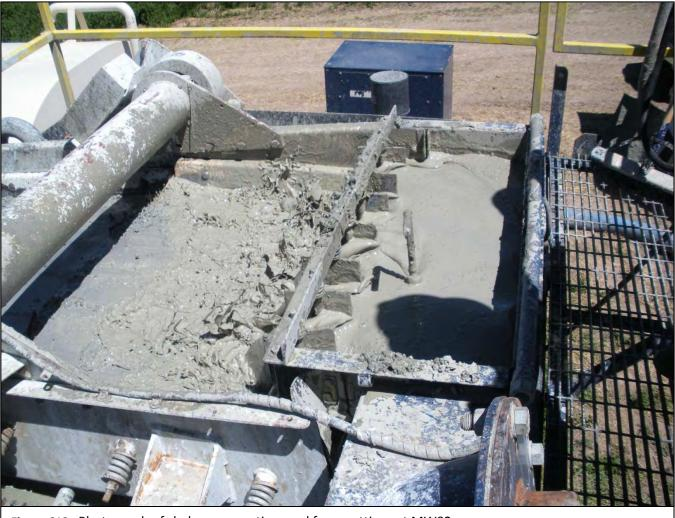
Figure C13. Photograph of shakers separating mud from cuttings at MW02.
