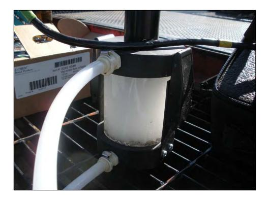
Figure D4. Photograph of water (foaming) flowing into YSI flow cell at MW02.
