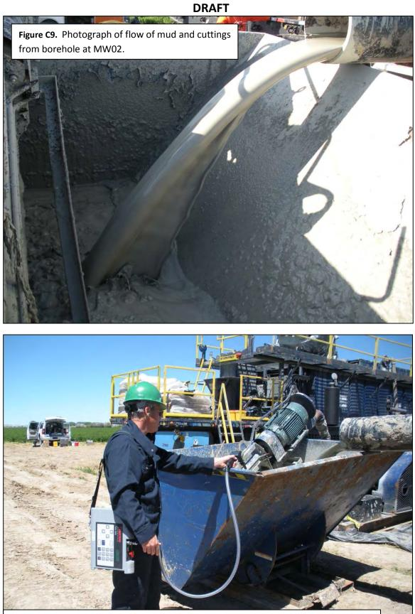
**Figure C10.** Photograph of monitoring of mud and cuttings using a Thermo Scientific TVA-1000B FID/PID at MW02.
