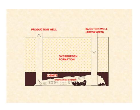
UCG is the insitu conversion of unworkable (deep seated, thin seam, steep dipping) coal/lignite into a combustible product gas.
