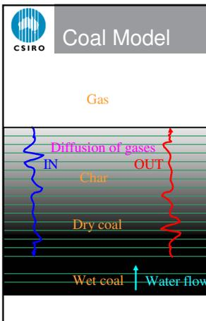
The coal model represents lump coal reacting with a hot gas.
