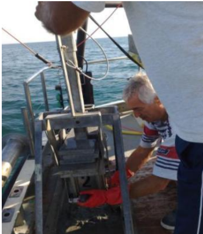
Box corer which was used to collect sediment samples for microphytobenthos and meiobenthos.
