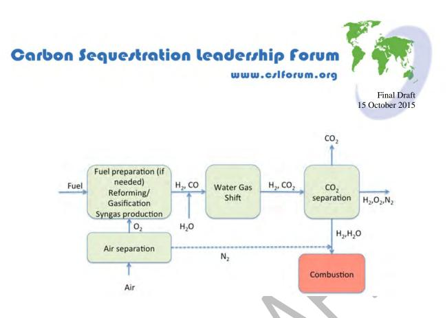
Figure 2. Schematic illustration of the pre-combustion process
