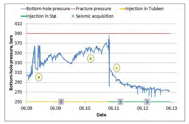
Figure 7-3 Pressure history at the Snøhvit CO<sub>2</sub> storage site (2008 to 2013) with time-lapse seismic acquisition surveys. Three main features of the injection pressure history are: a) early rise in pressure due to near-wellbore effects related to salt drop-out, b) a gradual rising trend in pressure due to geological flow barriers in the Tubåen Fm., and c) pressure decline to a new stable level following diversion of the injection into the overlying Stø Fm.
