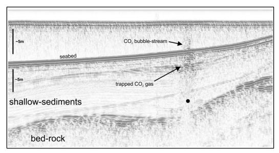
Figure 7-11 Seismic profile at the QICS site showing gaseous CO<sub>2</sub> trapped in shallow sediments and a bubble stream above the release point.
