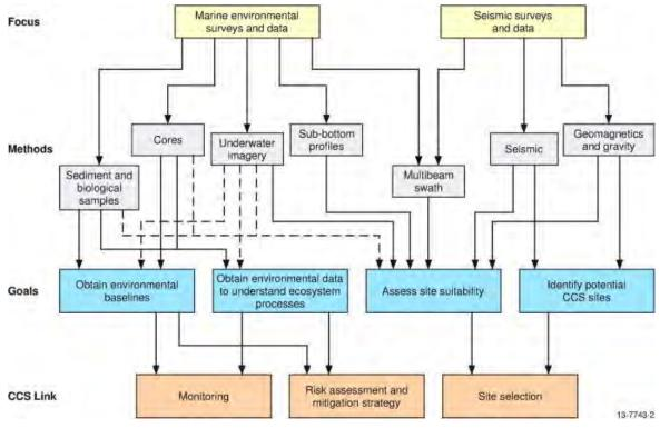
Figure 7-8 Diagram showing the roles of environmental (seabed and shallow sub-seabed) and deep geological (seismic) data to sub-seabed storage of CO<sub>2</sub>. Solid lines indicate likely relationships, and dashed lines indicate potential relationships.<sup>264</sup>
