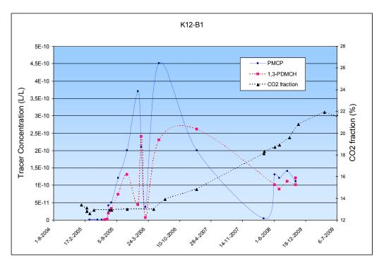
Figure 7-4 Tracer concentrations and CO2 fractions at the K12-B1 production well. Tracer concentration data for both tracers show tracer breakthrough after 130 days (August 2005) for the K12-B1 well and after 463 days for the 12-B5 well (June 2006).
