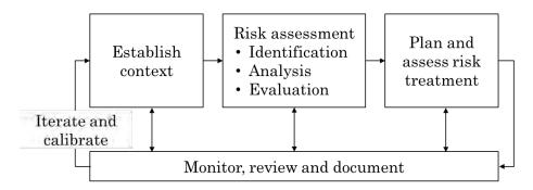
Figure 5-1. Recommended risk management process for CO<sub>2</sub> geological storage.<sup>1</sup> Risk assessment consists of risk identification (the process of finding, recognizing and describing risks), risk analysis (the process to comprehend the nature of risk and to determine the level of risk), and risk evaluation (the process of comparing the results of risk analysis with the risk criteria to determine whether the risk and/or its magnitude is acceptable and tolerable).
