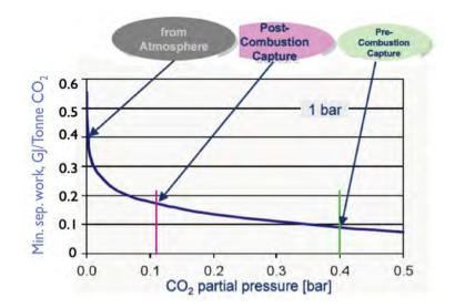
Figure 1: Theoretical minimum separation work of CO<sub>2</sub> from a flue gas depending on the partial pressure of CO<sub>2</sub> [modified from Bolland et al., 2006]
