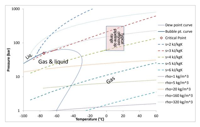
Figure 4-3: Typical phase diagram of natural gas within pipeline spec., including curves for constant  $(\rho)$  and entropy (s).
