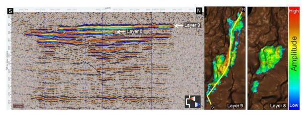
Figure 7-5 Time-lapse response (1994 to 2010). Left: seismic difference section, right: map view of the two uppermost layers.
