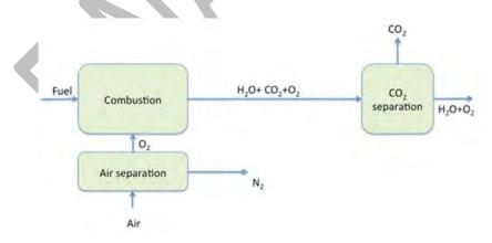
Figure 3. Schematic illustration of the oxy-combustion process
