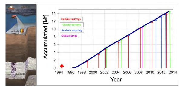
Figure 7-2 Illustration of seismic, gravimetry and sonar measurements at Sleipner (left) and monitoring techniques employed at Sleipner as a function of CO<sub>2</sub> stored (right)
