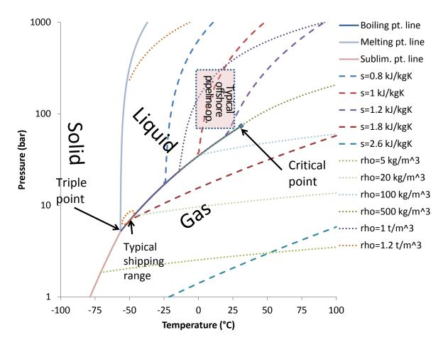
Figure 4-2: Phase diagram of pure CO<sub>2</sub>, including curves for constant density ( $\rho$ ) and entropy (s), calculated from the Span-Wagner equation of state.
