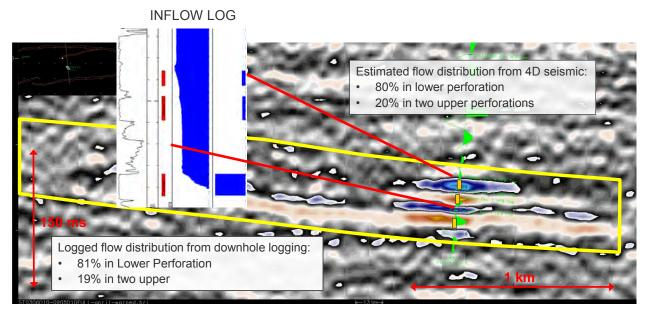
Figure 7-7 Comparison of downhole flow logging at the Snøhvit CO<sub>2</sub> storage site with flow distribution estimate from time-lapse (4D) seismic (yellow box indicates the Tubåen storage unit).
