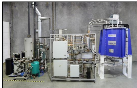
The VeloxoTherm™ demonstration unit, with all the features of a full plant, supports continuous quality-characteristic testing for endurance and reliability. Photo Credit: Inventys
