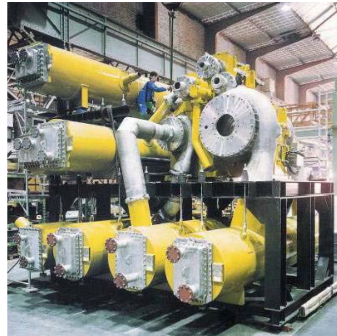
10-stage integrally geared centrifugal compressor
