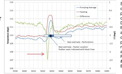
Successful diagnosis of pressure bleed off issue – i.e., DTS showed fluid influx above packer due to off depth perforations, not the MBM assembly (B Freifeld, LBNL & R Trautz, EPRI)
