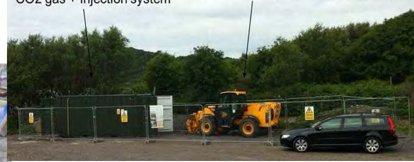
Telehandler for changing gas pallets
