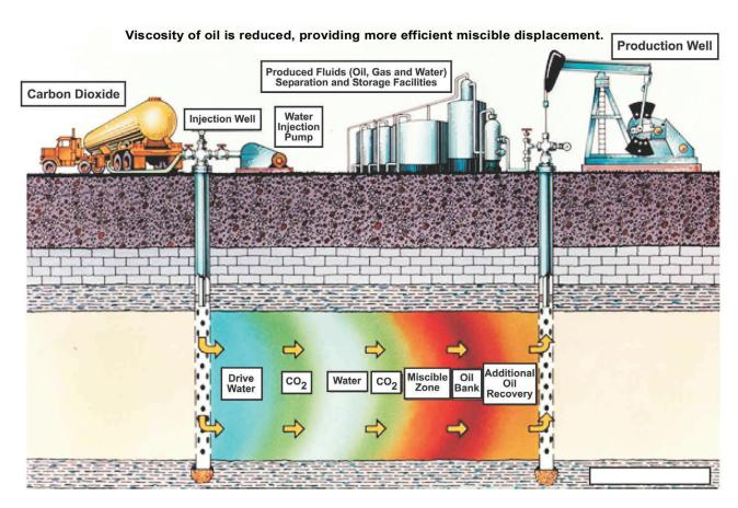
Cross-section illustrating how carbon dioxide and water can be used to flush residual oil from a subsurface rock formation between wells. Source: "Carbon Dioxide Enhanced Oil Recovery," U.S. Department of Energy, National Energy Technology Laboratory, March 2010, page 5.
