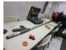
Borehole gravity meter being assembled
