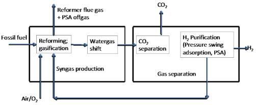
PSA offgas (H<sub>2</sub>, CO, CO<sub>2</sub>, CH<sub>4</sub>, N<sub>2</sub>++)
