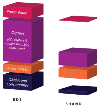
Figure A.2.1. Cost reductions for Shand 2 nd Generation CCS study relative to Boundary Dam Unit 3 Costs. Overall reduction of cost of capturing carbon on a per tonne basis is 67%, from [1,2].
