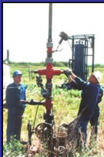
Single well injection test: Alberta Enhanced Oil-bed Methane Recovery Project
