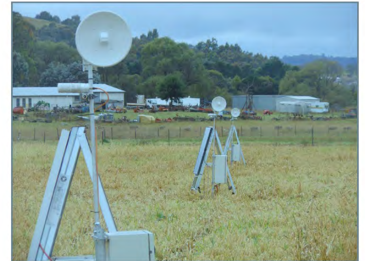
Fig. 1. Three of the sensor platforms, deployed at the Ginninderra test site near Canberra, Australia. The Vaisala GMP343 can be seen on the masts; power is provided by solar panels and all remaining equipment is securely housed in a box on the mast.
