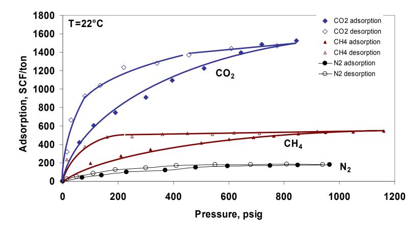
Substantially more  $CO_2$  adsorbs on coal particle surfaces than does  $CH_4$  or  $N_2$ . Once the  $CO_2$  is adsorbed, it will stay adsorbed even if pressure is reduced significantly.
