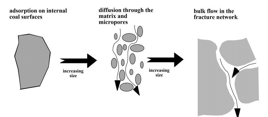
In many coal beds, methane is adsorbed on coal surfaces. When  $CO_2$  is injected, it replaces the methane, which can then be recovered.
