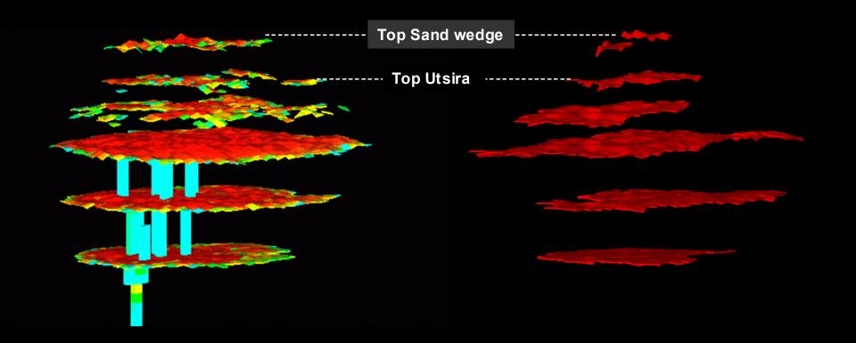
Gravity segregation with flow under shales strongly influences the distribution of injected  $CO_2$ .
