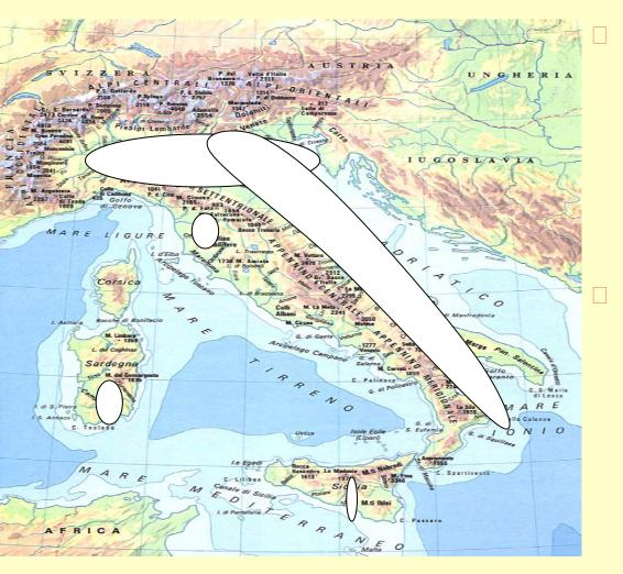
The saline aquifers, oil and gas depleted reservoirs, either on-shore or off-shore, are particularly well distributed in the Padanian back-arc basin and in the Adriatic see.
