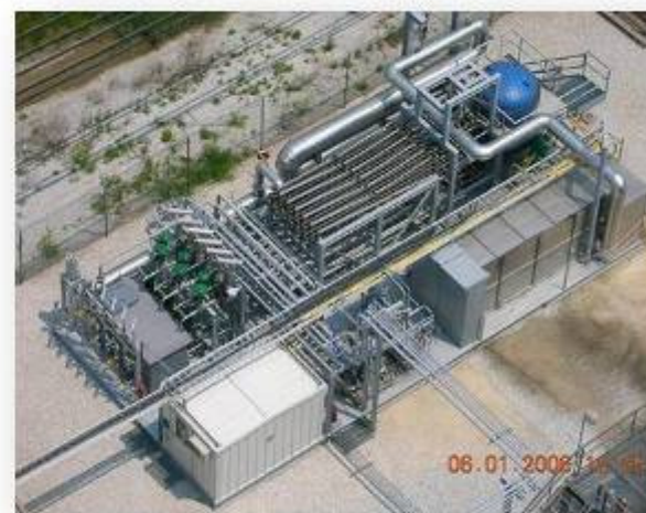
5 TPD Subscale Engineering Prototype (SEP) ITM Test unit at APCI's Sparrows Point gas plant
