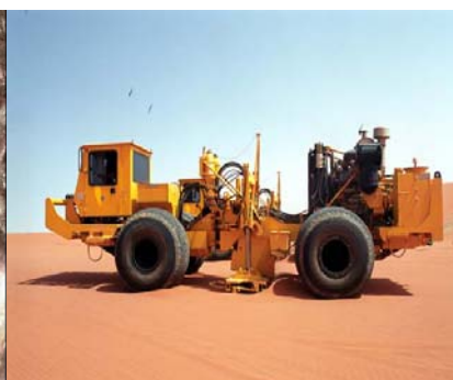
Seismic Source: Vibrosis Truck
