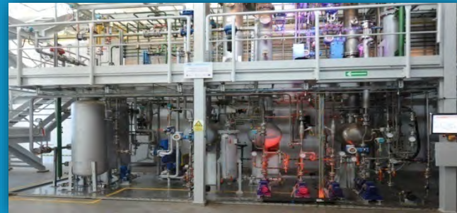
Installation for CO 2 separation, 100 m 3 /h
