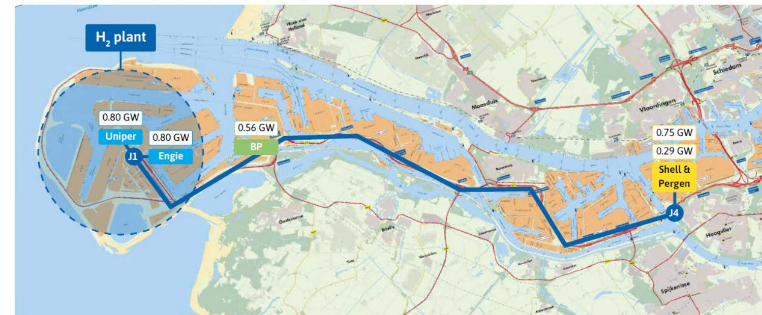
Figure 6.10: Reference scope case overview of the blue hydrogen production and transport infrastructure for the Rotterdam port, including both RFG and NG heating demand from end users. 'J#' are identifiers for junction points where the transmission pipeline splits into smaller lines going directly towards the plants.
