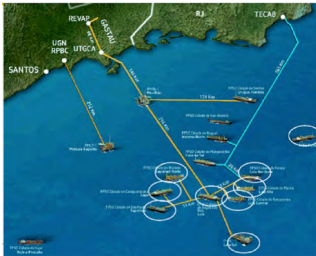
Figure 3. The network FPSOs with CO 2 separation and injection facilities for enhanced oil recovery (EOR) in the Santos basin, offshore Brazil. Courtesy: Grava, W.M. 2018. "Technology for Offshore Gas Production". The 4th Brazilian Congress on CO 2 in the Oil, Gas and Biofuels Industries, Rio de Janeiro.
