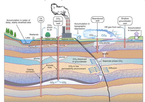
The objective of this effort is to develop a simple framework for evaluating leakage risk for certifying operation and decommissioning of geological CO<sub>2</sub> storage sites.
