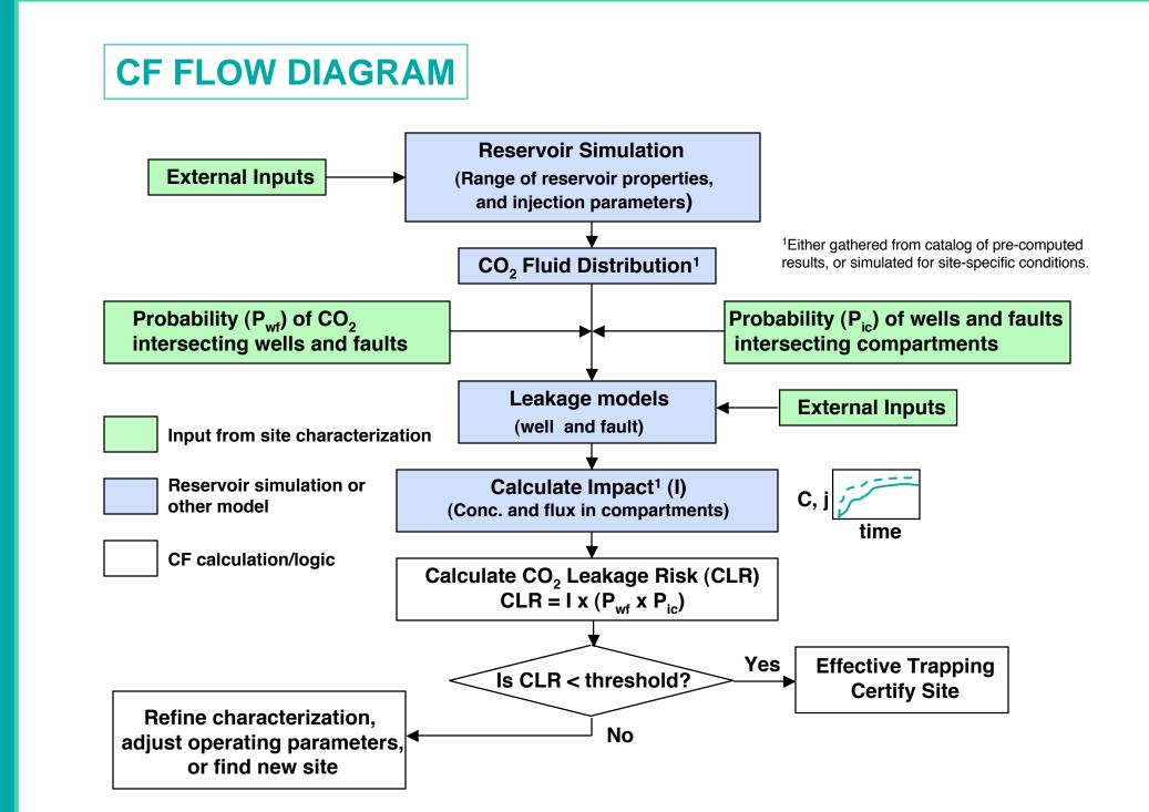
Reservoir Simulation is used to calculate CO<sub>2</sub> fluxes and concentrations with time in compartments. Fluxes and concentrations are either read from catalog of pre-simulated results or computed on a site-specific basis.
