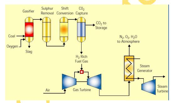
Figure 2. Coal-fired IGCC with pre-combustion capture of CO<sub>2</sub> (courtesy of the IEA Greenhouse Gas R&D Programme)
