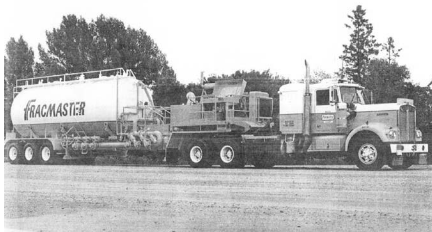
Figure 3. Liquid CO 2 from the truck and the solid proppant are mixed in a closed vessel and used for subsequent fracturing in the Dry-Frac stimulation. Source: Mazza, 2001
