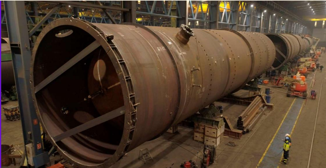
Fabrication of storage tanks by Idesa, Spain
