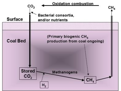
Figure 2. Enhanced CBM followed by microbial regeneration of the CBM reservoir.
