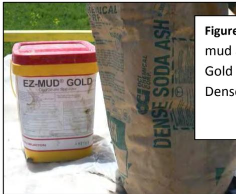
Figure C7. Photograph of mud additives EZ Mud Gold (Halliburton) and Dense Soda Ash.
