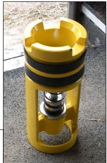
**Figure C3.** Photograph of blowout preventer for drillstem.
