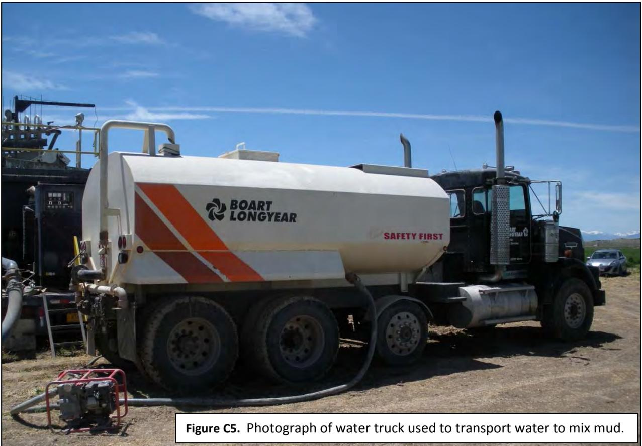
Figure C5. Photograph of water truck used to transport water to mix mud.
