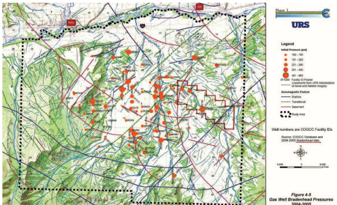
Figure 4. Map of distribution of reported initial bradenhead pressures of gas wells, mapped structural features and Mamm Creek Field Special Drilling Zone. Modified from URS (2006).
