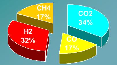
Calorific Value 2600 Kcal / sm<sup>3</sup> With no CO<sub>2</sub> capture Calorific Value 4000 Kcal / sm<sup>3</sup> With CO<sub>2</sub> capture
