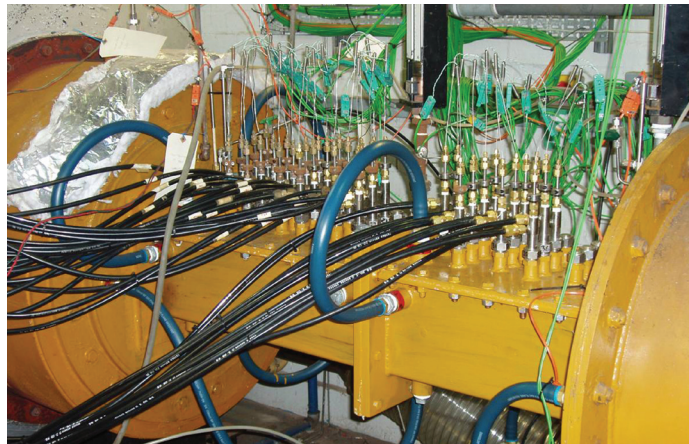
Cranfield University burner rig during first exposure period with materials probes installed.
