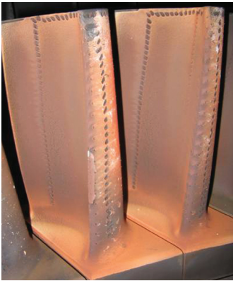
Blade from first stage of a used Siemens F class gas turbine showing thermal barrier coating and some of the cooling air exit holes
